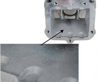
Cylinders marked 223994 and 223993 with linear texture in the inlet port show a fully CNC machined exhaust port and a fully CNC machined top edge of the central boost port.
