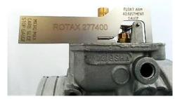
6.7.2 Needle valve assembly stamped "150".
