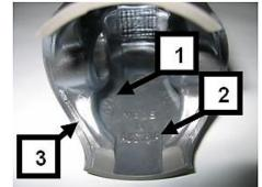
forbidden, if carbon is removed it must be consistently removed across the entire surface without altering the profile of the piston itself).
