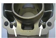
5.5.2.2 All ports have chamfered edges. Any additional machining is not permitted.
